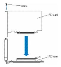
2. Align the riser with the slot on the logic board and press to seat the card.
